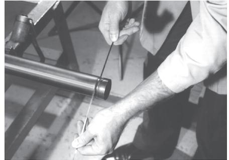
5. After a trial groove is prepared and the tool is removed from the pipe, carefully check the groove diameter (“C” dimension), as charted in the “Roll Groove Specifications” section. The “C” dimension is best checked with a pi-tape. It also may be checked with a vernier caliper or narrow land micrometer at two locations, 90° apart, around the groove. The average reading must equal the required groove diameter specification.
