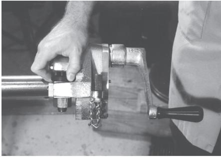
6. If the groove diameter (“C” dimension) is not within tolerance, the depth stop collar must be adjusted to obtain the proper dimension. To adjust for a smaller groove diameter, turn the depth stop collars **counterclockwise**. To adjust for a larger groove diameter, turn the depth stop collars **clockwise**. A quarter turn either way will change the groove diameter by 0.017 inch. A full turn either way will change the groove diameter by 0.068 inch.
