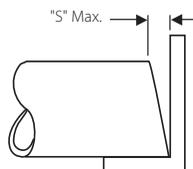
Any internal and external weld beads or seams must be ground flush to the pipe surface. The inside diameter of the pipe end must be cleaned to remove coarse scale, dirt, and other foreign material that might interfere with or damage grooving rolls. The front edge of the pipe end shall be uniform with no concave/convex surface features that will cause improper grooving roll tracking or result in difficulties during coupling assembly.
