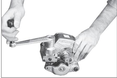
1. Using the crank, retract the upper roll arm fully by turning the feed nut counterclockwise.
