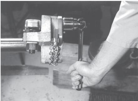
**5.** A ratchet with 1 1/4" socket (not supplied) may be used in place of the crank to operate the tool in low clearance conditions.
