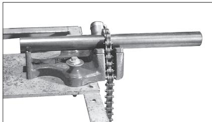
3. Secure a length of pipe/tubing in the pipe vise. Pipe/tubing position and pipe vise anchoring must be capable of handling the weight of the tool (17 pounds/8 kilograms), plus the manual effort required to operate the tool (approximately 20 ft-lbs/27 N•m of torque). Position the pipe/tubing to overhang the pipe vise by approximately 5–12 inches/125–300 mm, as shown, so that the tool can rotate freely.
