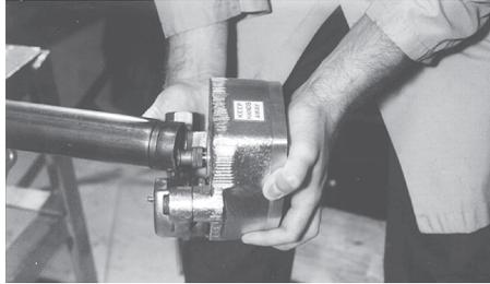
3. Lift the tool and remove it from the pipe.
