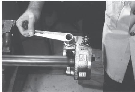
3. Advance the feed by turning the feed nut clockwise by the amount shown in the “Feed Rates” section. Feed rates for the VE12 vary depending on material and wall thickness.
