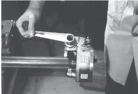
3. Using the crank, advance rolls together by turning the feed nut clockwise. Continue advancing until the grooving rolls are in light, but firm, contact with the pipe.
