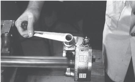
2. Turn the feed nut counterclockwise to retract the upper roll arm to the full open position.
