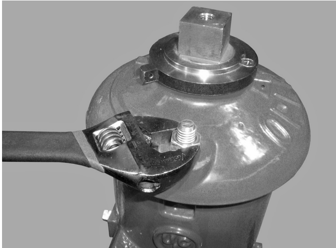
12. Re-install and tighten the two bolts/nuts.
